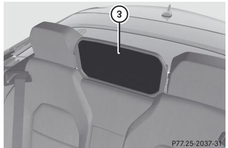
The head restraints on the rear bench seats and AIRCAP wind screen ③ move to the center position simultaneously.
