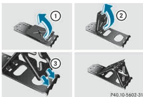
If your vehicle is equipped with a wheel chock, it can be found in the tire-change tool kit (▷ page 308).
