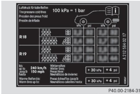
Some tire pressure tables show only the rim diameters instead of the full tire size, e.g. **R18**. The rim diameter is part of the tire size and can be found on the tire sidewall (▷ page 338).
