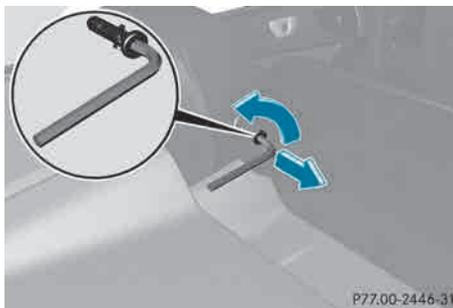
Bolts on the AIRCAP wind screen between the head restraints in the rear compartment
