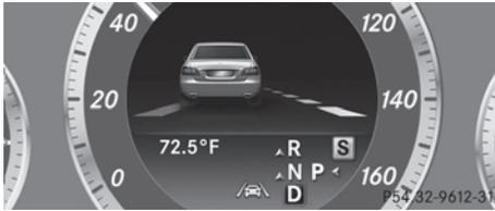
If a lane-correcting brake application occurs, the display shown in the illustration appears in the multifunction display.
