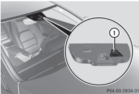
Lane Keeping Assist monitors the area in front of your vehicle by means of a camera ① at the top of the windshield. Lane Keeping Assist detects lane markings on the road and warns you before you leave your lane unintentionally.
