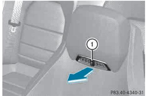
You can adjust the blower output of AIRSCARF vents ① using the AIRSCARF button (▶ page 112).
