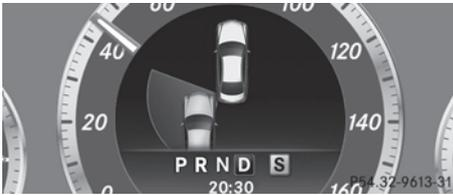
If Active Blind Spot Assist detects a risk of a lateral collision in the monitoring range, a course-correcting brake application is carried out. This is meant to assist you in avoiding a collision.
