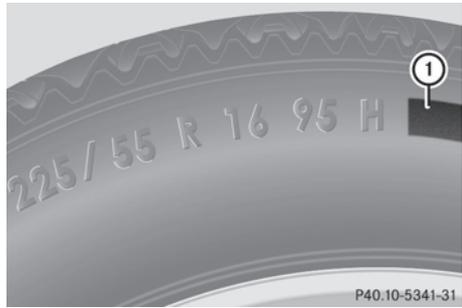
In addition to the load bearing index, load index ① may be imprinted after the letters that identify speed index ⑥ on the sidewall of the tire (▷ page 338).
