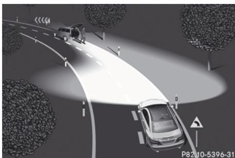
The active light function is a system that moves the headlamps according to the steering movements of the front wheels. In this way, relevant areas remain illuminated
