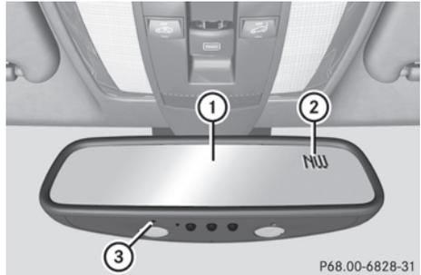
To receive a correct display in rear-view mirror ①, the compass must be calibrated and the magnetic field zone set.
