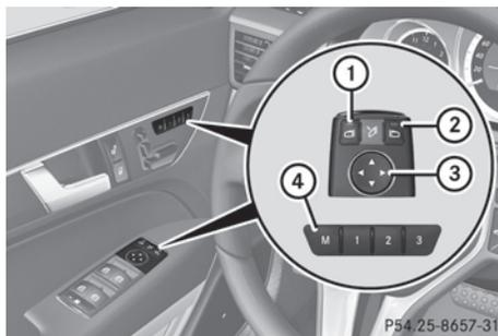
You can position the front-passenger side exterior mirror in such a way that you can see the rear wheel on that side as soon as you engage reverse gear. You can store this position.
