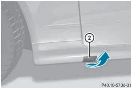
► **Vehicles with AMG equipment:** fold cover ② upwards.
