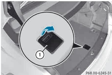
The TIREFIT kit, the vehicle tool kit, etc. are located in the storage compartment.
