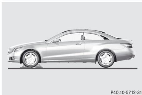
Securing the vehicle on level ground (example: Coupe)
